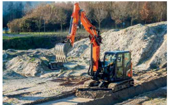
The optional floating angle blade is ideal for grading and levelling.
